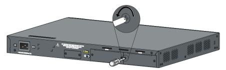
Figure 3-22 Install an interface module (1)
